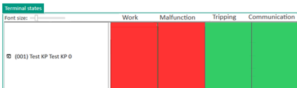
Figure 255 – Device is not ready for operation and there is a failure
